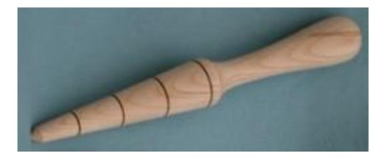
Wood required – 9" long by 1" diameter. Any hardwood, not too coarse grained would be suitable.
