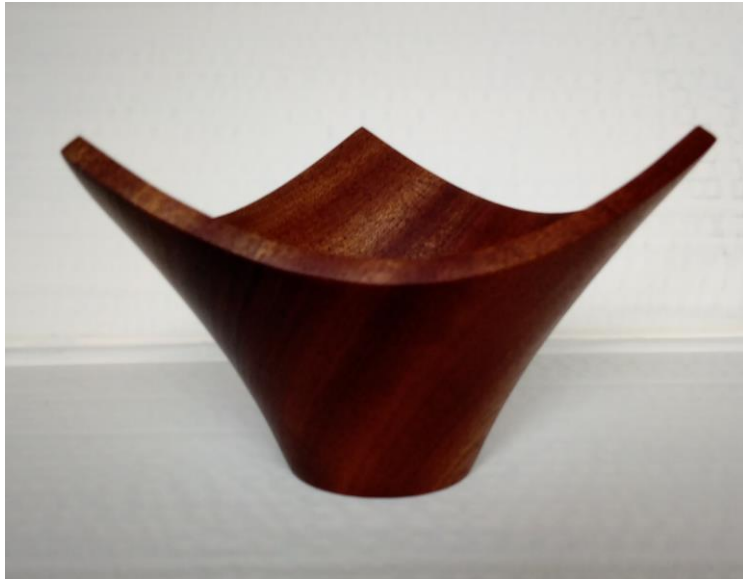
Demo piece finished as a simple bowl, Sapele with one coat of Osmo oil
